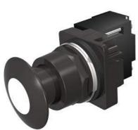
30mm BlackMax, Epoxy Coated Corrosion Resistant Complete Metal Unit Illuminated Push-Pull Operator Full Voltage, 6V AC LED Lamp Mushroom Head Cap Small 1 3/4" (44.5 mm) Metal, Black with White Lens 3 Position Pull-Momentary/Push-Maintained UL Listed, CSA Certified NEMA 1,3,3R,4,4X,12,13 & Automotive Standards
