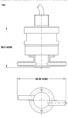
The Quick Calibration Hood is constructed from polypropylene, and provides a convenient means of supplying test gases to the IR600 in the field, for calibration and checking purposes. The assembly push-fits into the central gas access recess of the head, and is designed to accommodate 6 mm ID or 1/4" flexible tubing.
