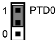
Figure 7-11: Accelerometer g-Select1 Jumper settings (J13)
