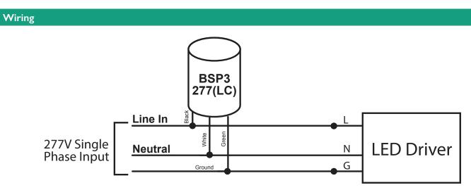
BSP3 and driver voltage must match input voltage
