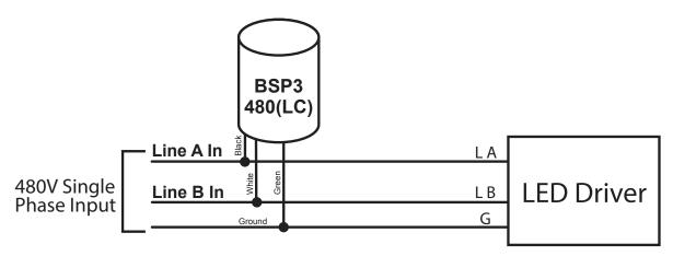
A single phase input from a 3-phase system uses only 2 phase line connections (A-B, B-L or C-A)
