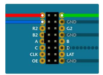
Pins R1, G1 and B1 (labeled R0, B0 and G0 on some matrices) deliver data to the top half of the display.
