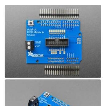
The shield comes with the button, terminal block, and the 16-pin header already soldered on. All you need to do is solder the headers!
