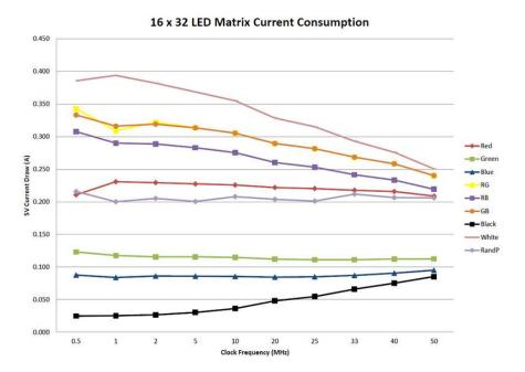
"Notice that the LED panel current consumption decreases as clock frequency increases. This suggests that the LED 'on time' is decreasing. I'm guessing this is caused by frequency-invariant delays in the LED driver shift registers."
