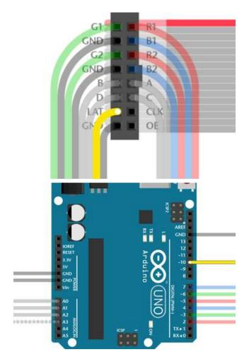
The LAT signal connects to Arduino pin 10.
