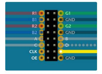
For 32x32 and 64x32 matrices, LAT connects to Arduino pin 10.
