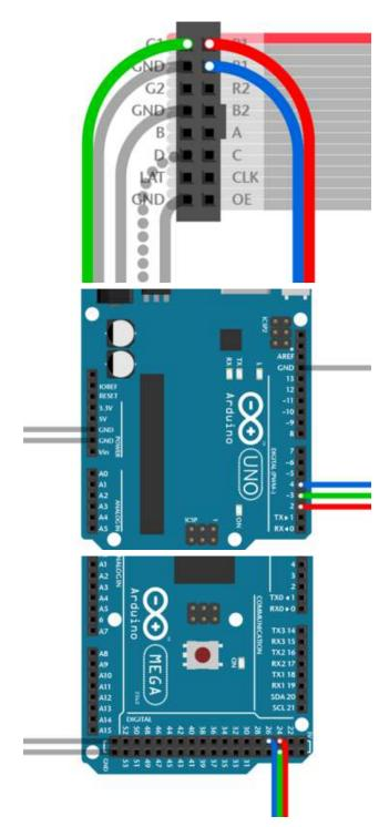
Pins R1, G1 and B1 (labeled R0, B0 and G0 on some matrices) deliver data to the top half of the display.
