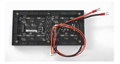
If your power cable came with spades at the opposite end of this power cable, they can be screwed into a 2.1mm terminal block adapter. Works nicely! Don't allow the exposed connectors to contact metal though...you should probably cover this with heat-shrink tube or electrical tape.
