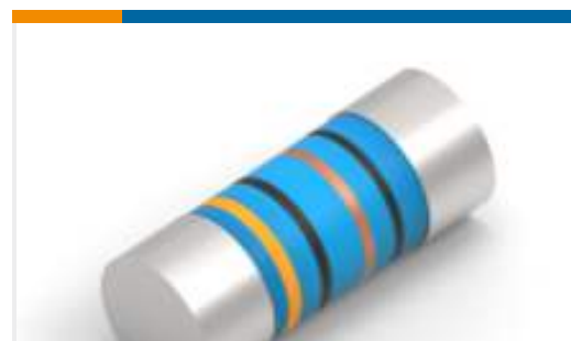
TE Part #3-2176316-7 MELF SMA_A 100K 0.1% 15PPM 0207 1W
