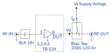
Fig 1. Block Diagram of Test Circuit used for characterization. (DUT soldered on Mini-Circuits Test Board TB-539+) Gain, Return loss, Output power at 1dB compression (P1 dB), Output IP3 (OIP3) and Noise Figure measured using Agilent's N5242A PNA-X microwave network analyzer.
