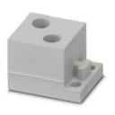
Cable sleeve, small, no. of conductors: 2, type: Round cable, slotted, external cable diameter: 2x 6.4 mm ... 6.7 mm, material: SEBS (halogen-free), color: gray, length: 29.5 mm, width: 19.5 mm, height: 17 mm
