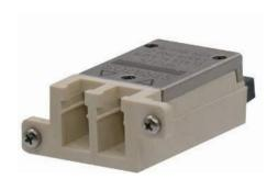
The FNK-ST11 multimode optical fiber transceivers provide low profile, cost effective solutions for Gigabit Ethernet and 1x Fiber Channel optical fiber data links with a duplex LC connector interface. These transceivers are fully compliant with the IEEE Gigabit Ethernet and ANSI 1x Fiber Channel standards but can be used for any other data communications purpose within their operating parameters.
