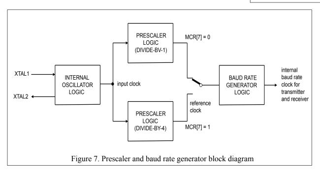
DLL and DLH must be written to in order to program the baud rate. DLL and DLH are the least significant and most significant byte of the baud rate divisor. If DLL and DLH are both zero, the UART is effectively disabled, as no baud clock will be generated.
