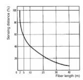
**Fiber Units with Reflective** Sensors (Fiber length of 2 m corresponds to 100%)
