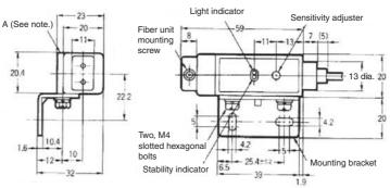
Note: The Mounting Bracket can also be used on side A.
