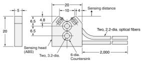
**Note:** The fiber for the emitter is identified by a white line.
