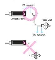
• Do not apply excess force on the Fiber Units.
