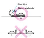
• The Fiber Head could be broken by excessive vibration. To prevent this, the following is effective:
