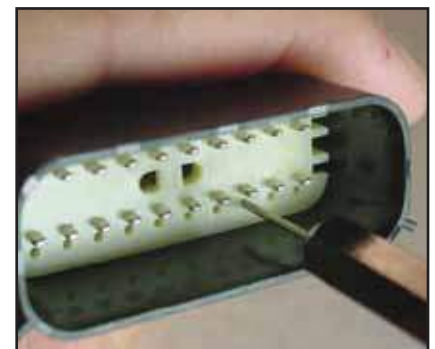
Service Tool must be 90° to the connector face
