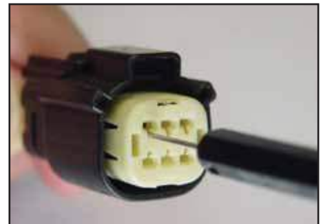
Service Tool must be 90° to the connector face
