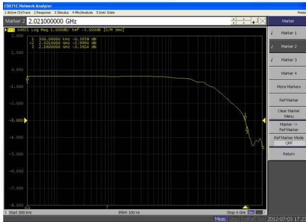
Figure 17. MHL Path SDD21 Insertion Loss Curve
