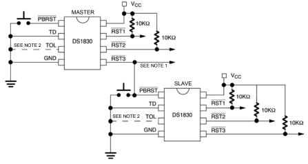
**Note 1:** The  $\overline{\text{RST3}}$  output tied to the pushbutton reset would be pulled to  $V_{CC}$  through the  $40k\Omega$  resistor in the pushbutton input. If a stronger pull-up is required an additional pull-up resistor could be added.
