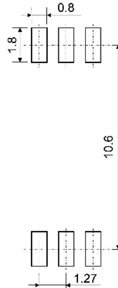
Fig. 15.2 Lead Forming Option (LF4)
