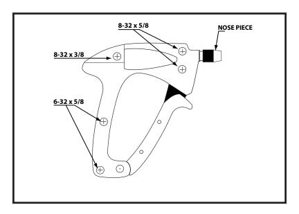
Turn the gun over and lay it down on a flat surface so the nose piece is facing left. Separate the housings and remove the collet and nose piece. Note: Use a flat head screwdriver to separate the housings.  Apply grease to the bevel, spur and face gear.
