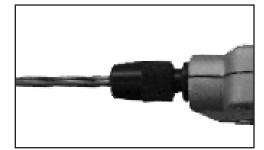
Place sleeve over the bit and slide the sleeve into the nose piece. Rotate the sleeve as you are sliding the sleeve into the nose piece until the sleeve has engaged with the collet pin, the sleeve will then slide further into the nose piece. The sleeve is now seated.
