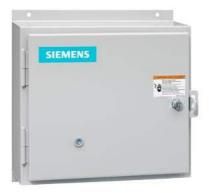
Non-reversing motor starter, Size 0, Single phase full voltage, Solid-state overload relay, OLRelay amp range 3-12a, 208VAC 60HZ coil, Non-combination type, Enclosure type 12, Dust/drip proof for indoors, Standard width enclosure
