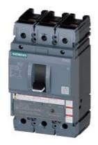
circuit breaker 3VA5 UL frame 250 breaking capacity class M 35kA @ 480 V 3-pole, line protection TM210, FTFM, In=150A overload protection Ir=150A fixed short-circuit protection Ii=10 x In UL489 SB (naval), 50 deg. cel. nut keeper kit on both sides
