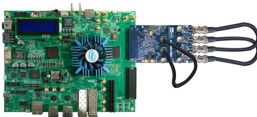
Figure 4-5 Hardware setup of SDI-FMC with A10SoC
