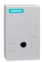
Non-reversing NEMA contactor, Size 1, Three phase full voltage, Contactor amp rating 27A, 3 wire (NO aux included), 208VAC 60Hz coil, Non-combination type, Enclosure NEMA type 1, Indoor general purpose use, Standard width enclosure
