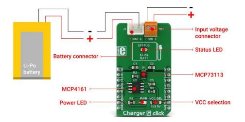
If a Li-Ion battery is discharged to below 3V, it has to be pre-charged with around 10% of the full charge current. This means that the charging current, in this case, will be 10% of the fast charging current set by the MCP4161 digital potentiometer.
