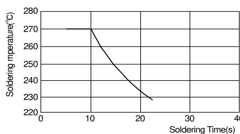
[Allowable Flow Soldering Temperature and Time]
