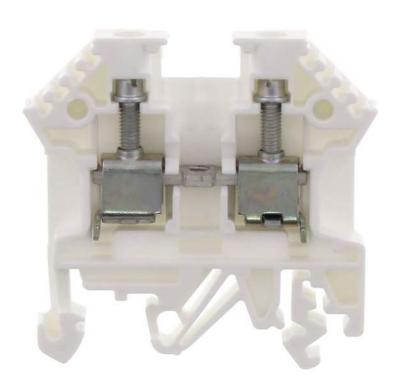
Feed-through terminal, Screw connection, Mounting type:Mounting rail TS 35/7.5 and TS 32, Rated cross-section: 4 mm², Width: 6 mm, Colour: White
