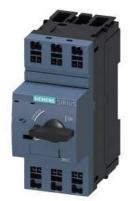
Circuit breaker size S00 for starter combination Rated current 3.2 A N release 42 A Spring-type terminal Standard switching capacity
