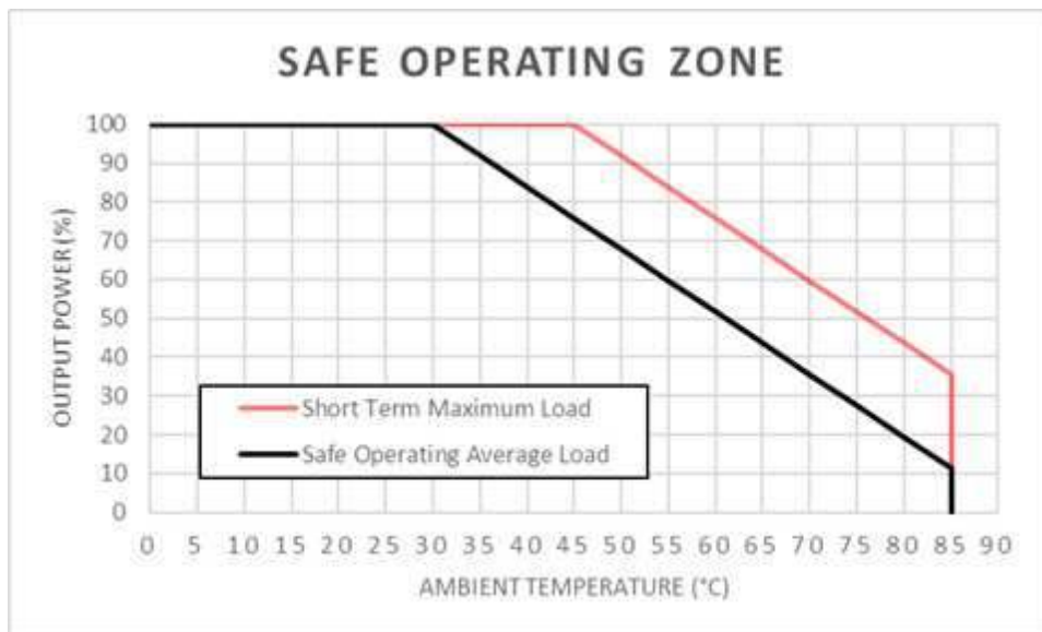
Figure 11 - Typical Application Derating Curve
