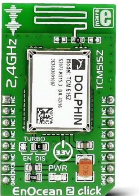
**EnOcean 2 click** carries the TCM 515Z transceiver, based on the **2.4 GHz IEEE 802.15.4** radio standard. The click is designed to run on a 3.3V power supply. It communicates with the target microcontroller over UART interface.
