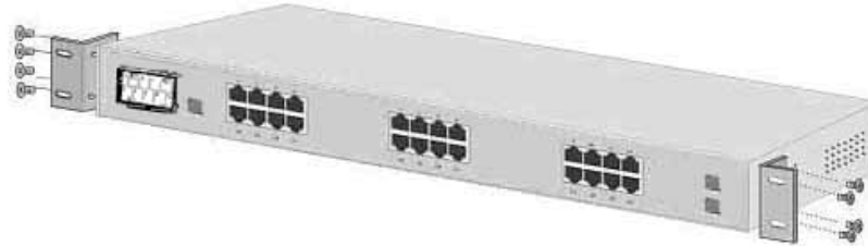
Figure 2.2: Attach mounting brackets with screws
