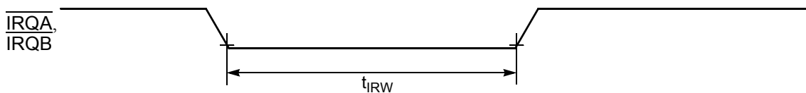
Figure 10-7 External Interrupt Timing (Negative Edge-Sensitive)
