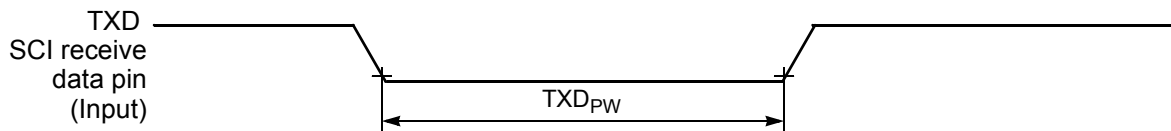
Figure 10-18 TXD Pulse Width
