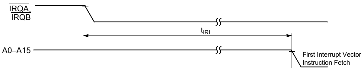
Figure 10-9 Interrupt from Wait State Timing
