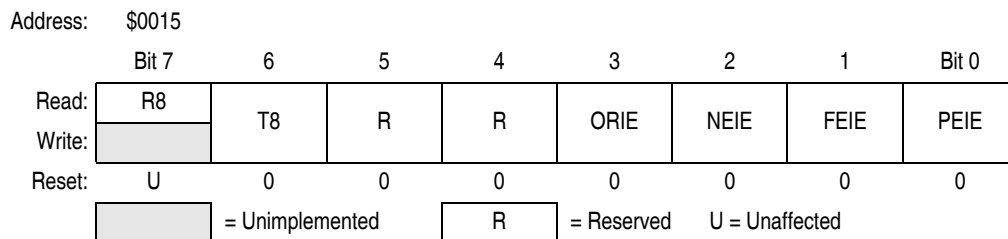
Figure 13-12. ESCI Control Register 3 (SCC3)
