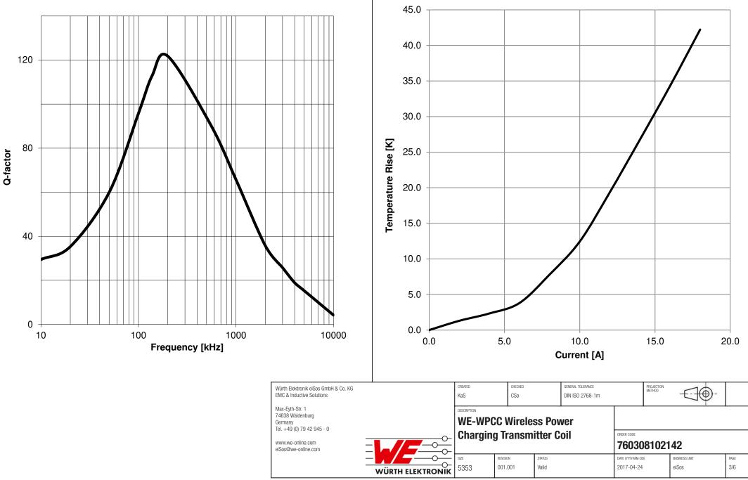
**Typical Temperature Rise vs. Current Characteristics:**
