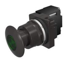
30mm BlackMax, Epoxy Coated Corrosion Resistant Complete Metal Unit Illuminated Push-Pull Operator Full Voltage, 120V AC/DC LED Lamp Mushroom Head Cap Small 1 3/4" (44.5 mm) Metal, Black with Green Lens 3 Position Pull-Momentary/Push-Maintained UL Listed, CSA Certified NEMA 1,3,3R,4,4X,12,13 & Automotive Standards
