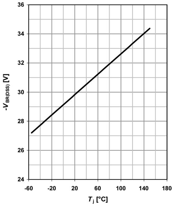
**28 Drain-source breakdown voltage (N)**
