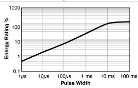
Published energy rating is for 10ms pulse. For shorter pulses energy rating has to be derated according to Max. Individual Pulse Rating chart and Single Pulse Energy Rating in TFSS consideration.
