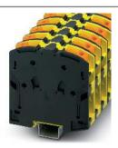
High-current terminal block, nom. voltage: 1000 V, nominal current: 232 A, connection method: Power-Turn connection, 1 level, cross section: 25 mm² - 95 mm², mounting type: NS 35/15, color: black/yellow
