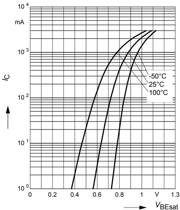
**Collector current  $I_C = f(V_{BE})$**
