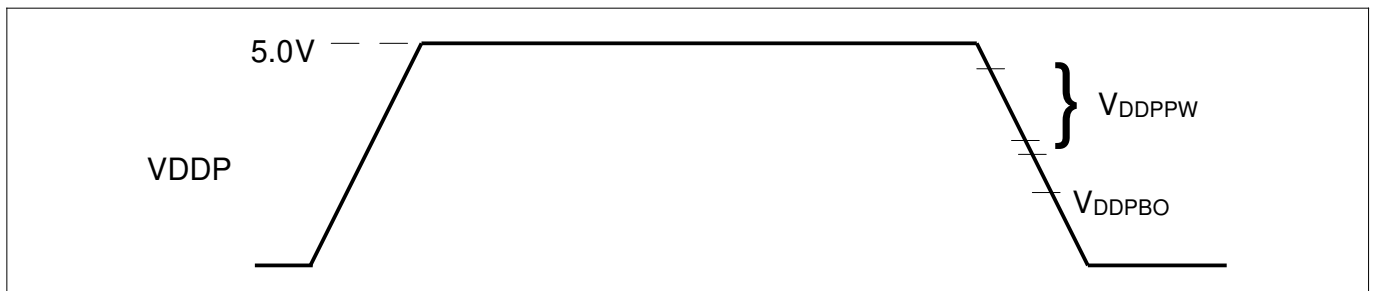
Figure 13 Supply Threshold Parameters
