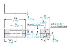
Material: Cold rolled carbon steel (SPCC)(Nickel plated)
