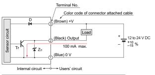
D: Reverse supply polarity protection diode Symbols ... ZD: Surge absorption zener diode Tr : NPN output transistor
