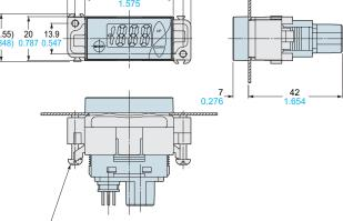
Two M3 (length 15 mm 0.591 in) screws for fitting are attached.
