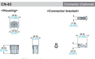
Mating connector Connector pin: BXA-001T-P0.6 manufactured by J.S.T Mfg. Co., Ltd. Housing: XAP-03V-1 manufactured by J.S.T Mfg. Co., Ltd.
