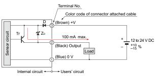
Symbols ... D : Reverse supply polarity protection diode ZD: Surge absorption zener diode Tr : PNP output transistor
