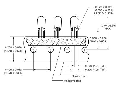
**Tape and Reel Specifications:** type 299D radial-leaded tantalum capacitors are available taped and reeled per EIA-468.
