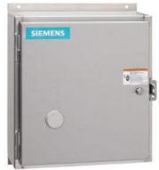
Mechanically held lighting contactor, Contactor amp rating 20Amp 0NC - 10NO poles, 265-277V 50/60HZ coil, Non-combination type, Encl NEMA type 4X 304 S-steel Water/dust tight noncorrosive
