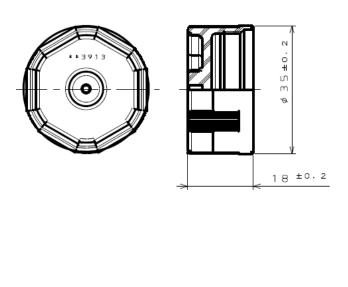
■ Waterproof Cap for Receptacle (with wire rope):
