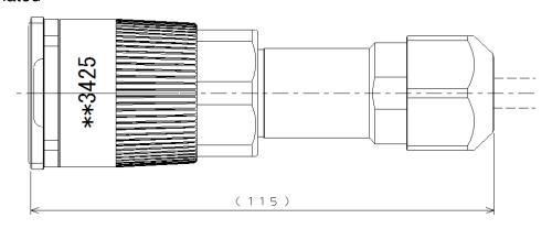
■Waterproof Cap for Receptacle (without wire rope):
