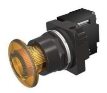
30mm BlackMax, Epoxy Coated Corrosion Resistant Complete Metal Unit Illuminated Push-Pull Operator Transformer type, 240V AC Incandescent Lamp Mushroom Head Cap Small 1 3/4" (44.5 mm) Plastic, Amber 3 Position Pull-Momentary/Push-Maintained UL Listed, CSA Certified NEMA 1,3,3R,4,4X,12,13 & Automotive Standards
