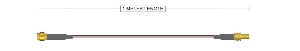
Connector A 132114RP SMA Plug Straight Brass Gold + Heatshrink 50 Ohm RG-316 Continuity/Hi-Pot Connector B 142189 SMB Jack Straight Brass Gold + Heatshrink
