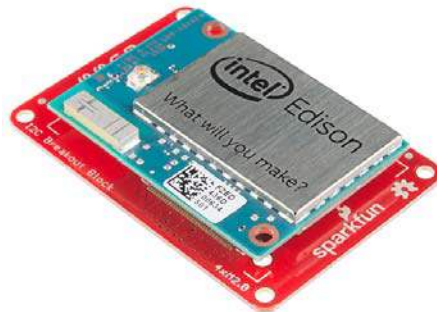
I2C Block Installed
