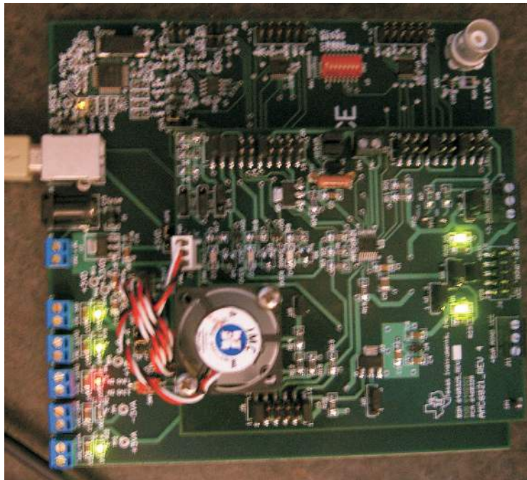
Figure 11. AMC6821EVM and USB-MODEVM Hardware Setup
