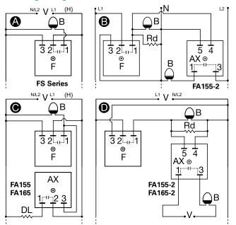
V = Voltage N = Neutral B = BeaconDL = Dummy Load for Constant Line Loading
