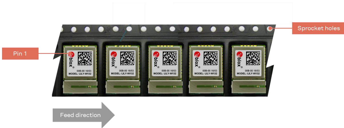
Figure 7: Orientation of LILY-W132 modules on tape
