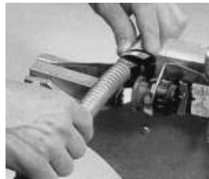
Cut through the helix with pliers
