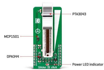
The voltage reference(VREF) is obtained from the MCP1501, a high-precision voltage reference IC from Microchip. The main purpose of this IC is to provide and retain a very accurate voltage of 4.096V. Its voltage reference is accurate enough for most applications where the analog output from the Slider 2 click can be utilized as a control voltage signal (CV). The output is
