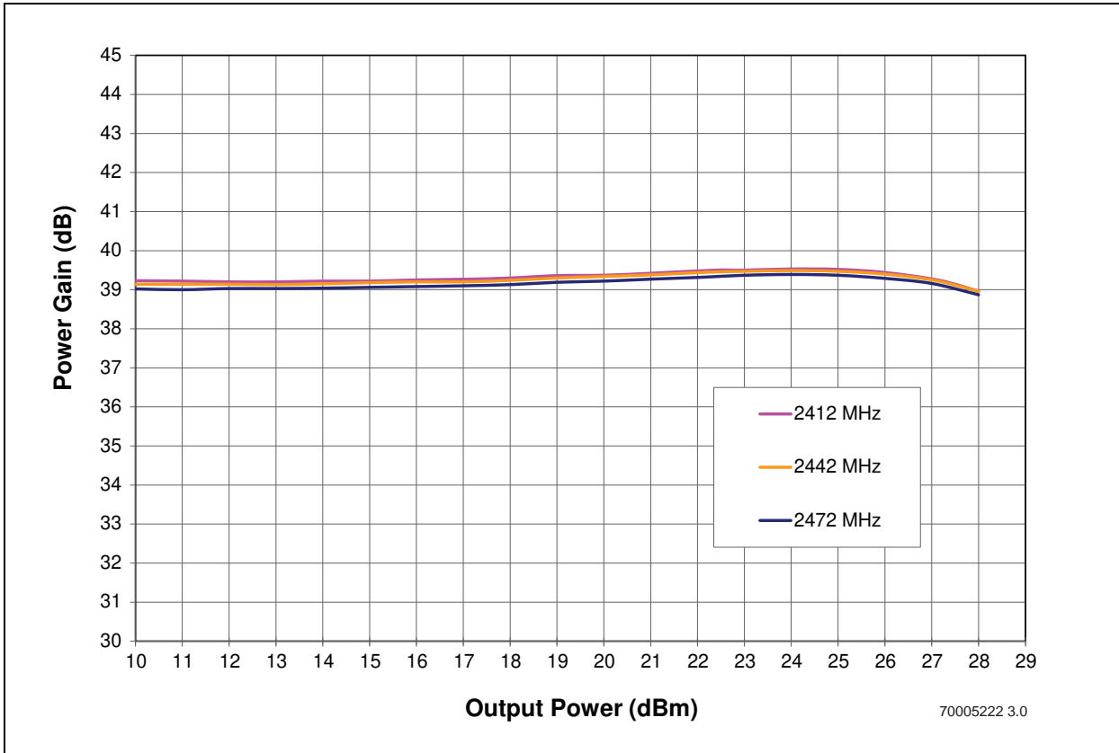
FIGURE 5-4: POWER GAIN VERSUS OUTPUT POWER
