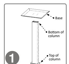
To secure base to column, turn column upside down (with top plate down) and place base inverted, as shown, on column.
